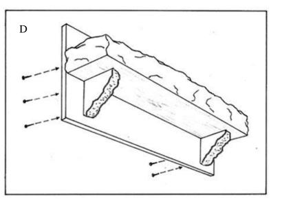
Square brackets need to be installed before the stone or brick facing is put up. The bracket recesses into the stud wall and is normally screwed or lagged to the side of a stud as shown in Figure E at right.
