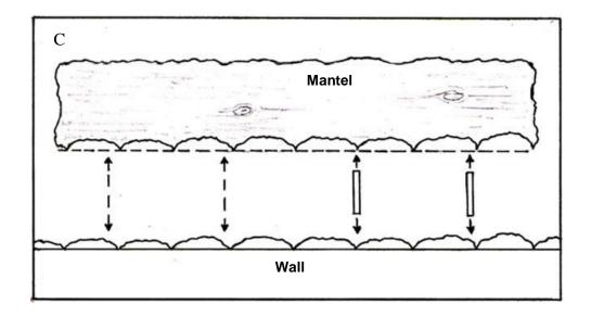
Please note, if the stone face of your fireplace is irregular, the back edge of the mantel can be scribed to fit the stone as shown in the diagram. The dotted line on the mantel shows the square back of the mantel as shipped, and the solid line shows the scribing to match the stone shape. The fit does not need to be perfect to look good, but it may take a few tries to match the mantel to the stone.
